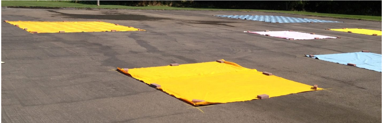
Figure 4. Image of the unmixing targets. The yellow/yellow unmixing target is in the upper left while the blue unmixing target is in the upper right. Four of the whole pixel targets are shown in the foreground.
