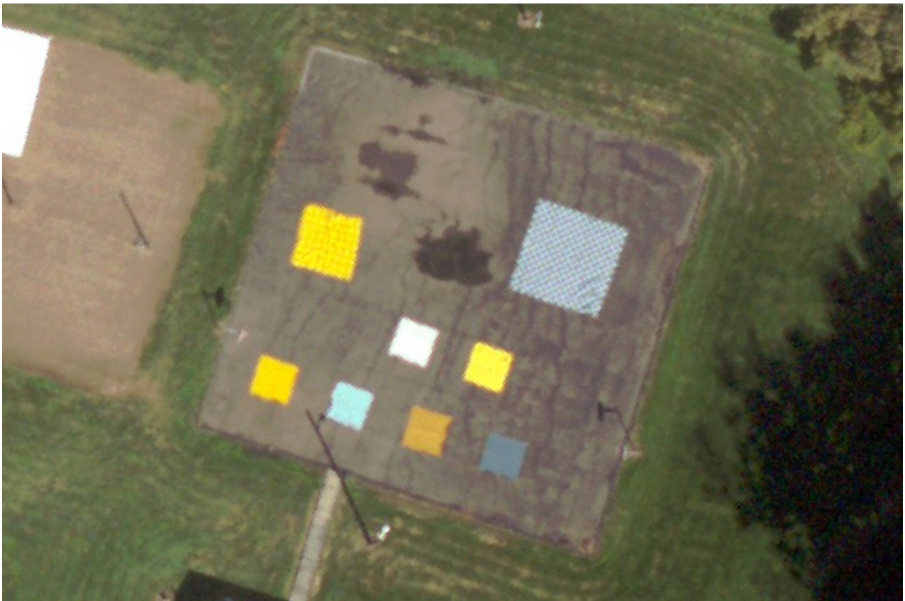
Figure 5. Unmixing target detection experiment deployment in the morning configuration. The large (24' x 24') 50/50 blue target is visible in the upper right area of the asphalt court while the smaller (16' x 16') 75/25 yellow/yellow target is in the upper left. The six 10' x 10' whole panels of the fabrics are seen clearly just below the unmixing targets. The two small panels just below and to the left of the blue target are pink felt (on the left) and yellow cotton (on the right). The four small panels across the lower part of the asphalt area are (from left to right): yellow felt, blue cotton, gold felt, and blue felt. The image is extracted from RIT WASP imagery collected at 1551Z with approximately 6" resolution.
