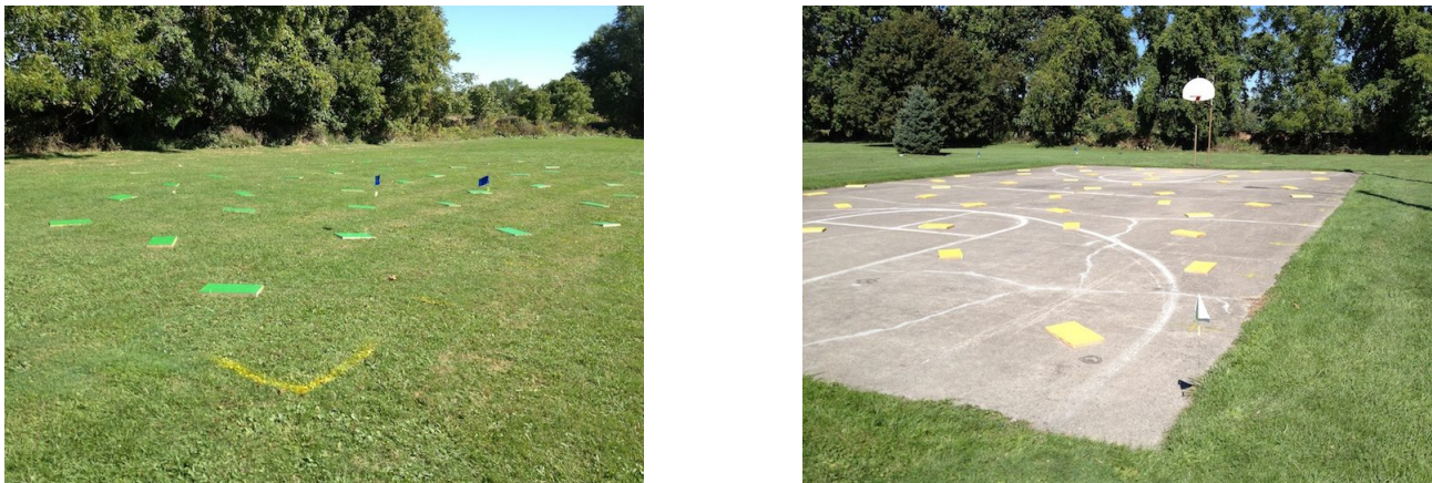
Figure 1. Subpixel targets. The green wooden blocks are shown in the grass field on the left while the yellow wooden blocks are on the right.
