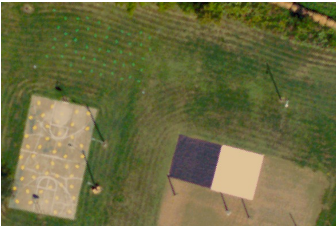
Figure 2. Subpixel target detection experiment deployment. The green wood blocks are seen in the grass in the upper left area of the image while the yellow wood blocks are seen on the basketball court in the lower left area of the image. The image is extracted from RIT WASP imagery collected at 1551Z with approximately 6'' resolution.
